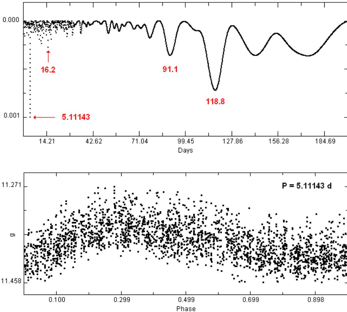
Figure 11: Periodogram obtained with *AVE* (upper panel) and light curve, in phase, plotted with ASAS-SN data using a period equal to 5.11143 days (lower panel): it appears moderately coherent with an amplitude equal to 0.187 magnitude.
